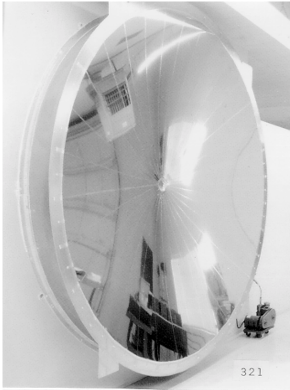
3 m diameter HAIR reflector (on-axis)
