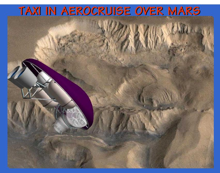
10 crew, Earth / Mars aerocapture, 12 m diameter aeroshell (Elliptical Raked Cone), 16.1 mt vehicle dry
