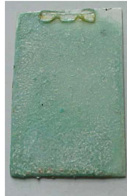
Copper Sheet with Integrated Piezoelectric/Solid Electrolyte Coating
