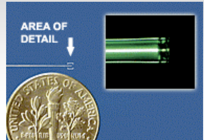
High temp. pressure sensor. 125 microns diam.
