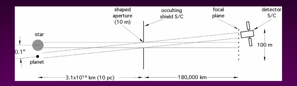
Large Distance Set by 0.01 arcsec requirement diffraction:  $\lambda/D = .01$ "  $\rightarrow D = 10m$  @500nm geometric: F = D/tan(.01") = 180,000km
