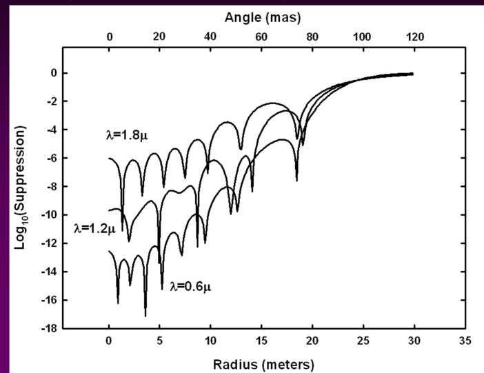
Suppression of Edge Diffraction Can Be Understood Using Fresnel Zones and Geometry
