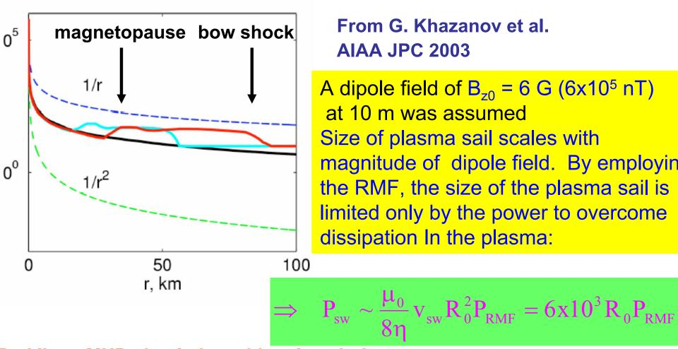
Red line - MHD simulation with solar wind
