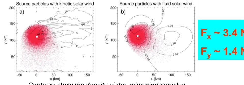
Contours show the density of the solar wind particles Source particles are indicated in red.
