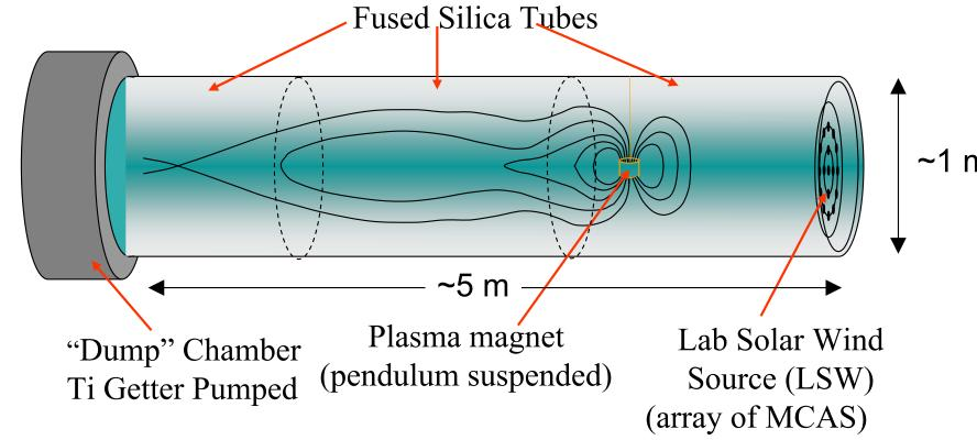
Want to maintain plasma magnet size with smaller antenna to observe expansion Against Laboratory Solar Wind (LSW)  $D_{Antenna} \sim 1/4 (0.4 \text{ m}) - 0.1 \text{ m}$
