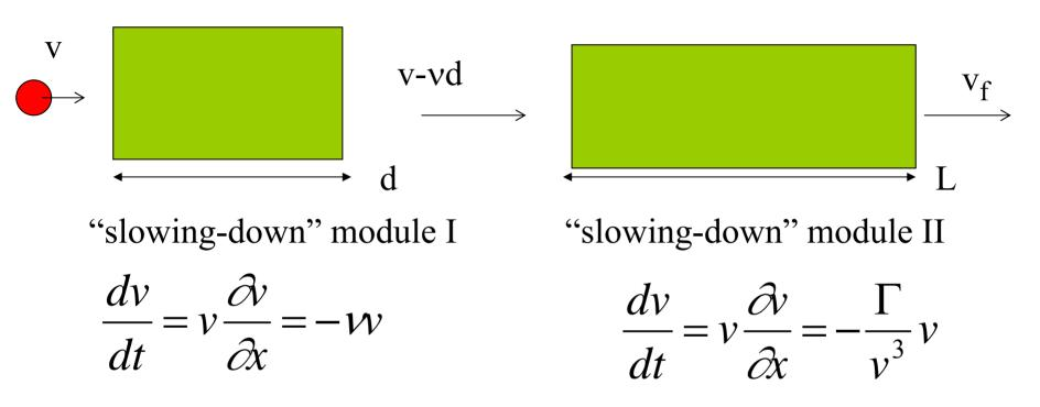
Particles coming from left suffer small slowing down in module I which results in large slowing down in module II, if  $v_f(v-vd,L)\cong 0$ .
