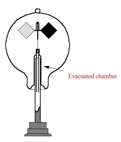
Depending on how "evacuated" the chamber is, the radiometer spins one way or the other
