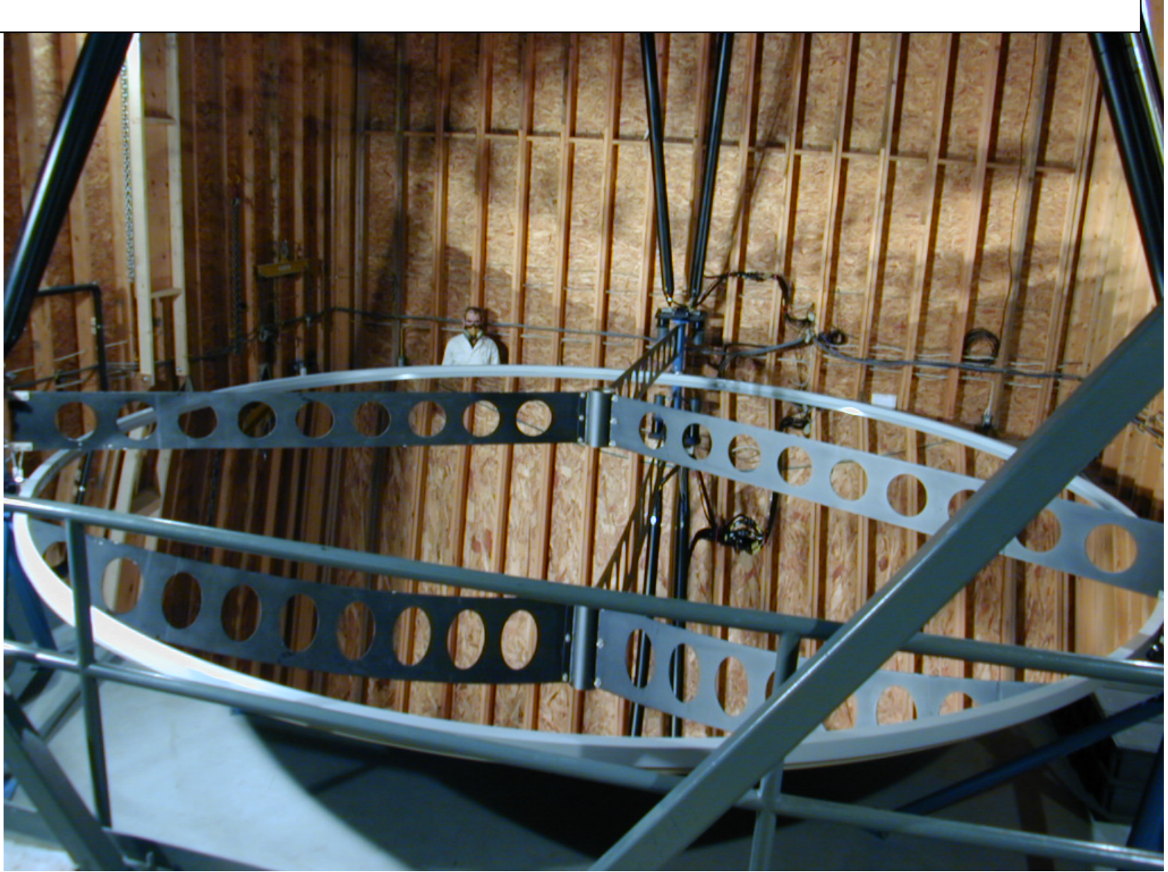
The 6 m diameter mercury liquid mirror of the LZT (courtesy P. Hickson)
