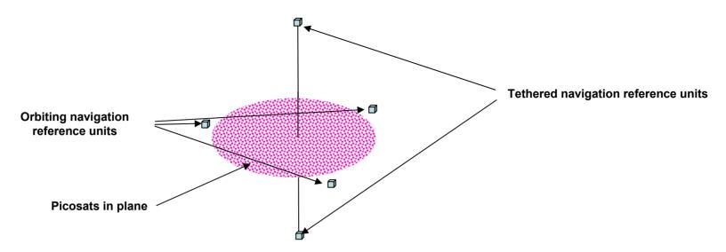
•Set up a GPS-like local navigation environment: a CMS (Constellation Metrology System) •5 reference units have stable oscillators and low power (short range) transmitters •Each picosat determines its own position, and then computes its required phase delay
