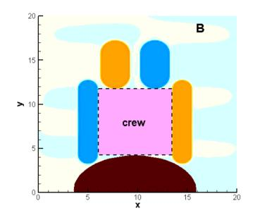
Contours of the calculated magnetic field created by a system of 4 coils. Dark region at the bottom resembles space craft, to which the habitat is attached.
