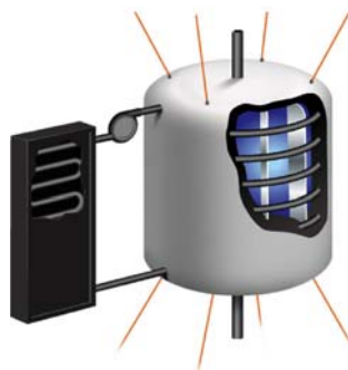
Zero-Boil-Off Cryogen Storage
