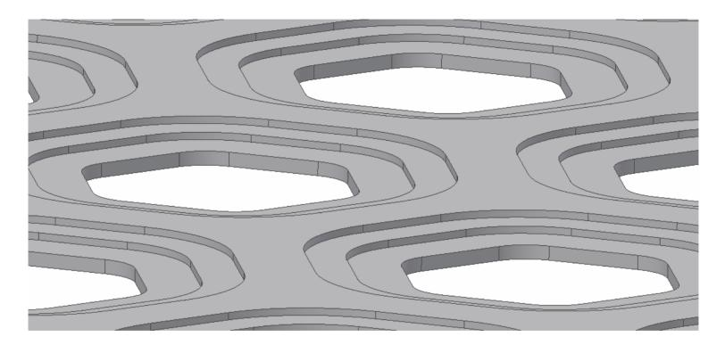
Holes are on 15  $\mu$ m centers maximum thickness 1.06  $\mu$ m Transmits 10% for full solar spectrum
