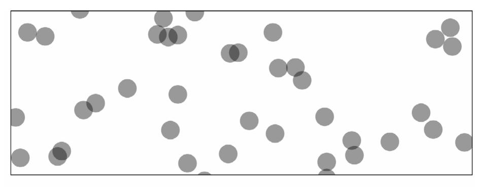
6% self-shadowing and 6% efficiency loss from being spread-out
