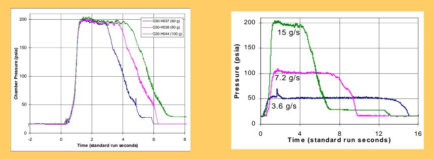
Pressure Curves for SCH<sub>4</sub>/GOX Firings, Showing Effect of Grain Size and Varying Oxygen Flow Rate
