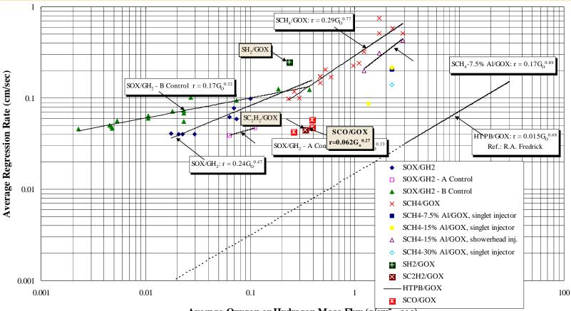
Average Oxygen or Hydrogen Mass Flux (g/cm<sup>-</sup> - sec)
