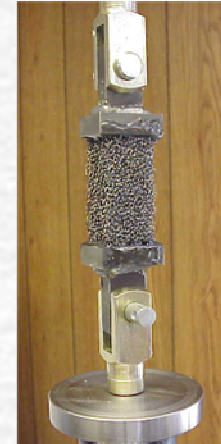
Open-Cell Structure and Tension Test Set-Up
