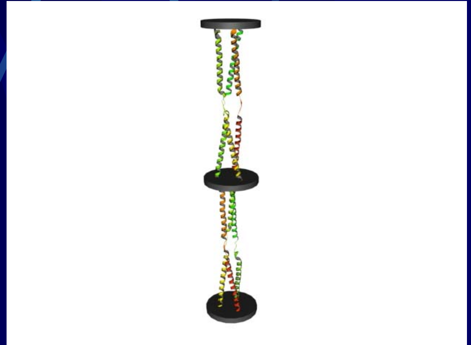
VPL Motors in Series – Displacement Multiplication
