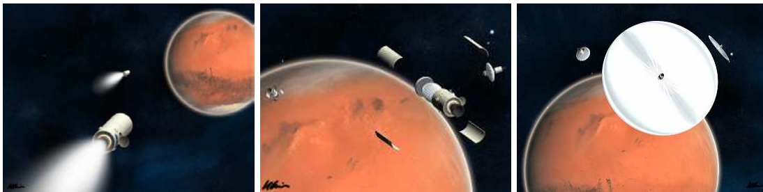
Fig. 26 Shows the LDR package approaching Mars (left), deploying (center) and fall into HEPO orbit fully deployed (right).
