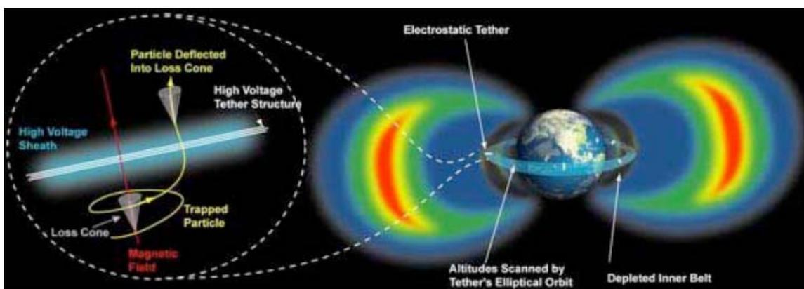
*Figure: Concept of operations of an electrostatic system deployed to reduce radiation fluxes in the inner electron Van Allen belt.*
