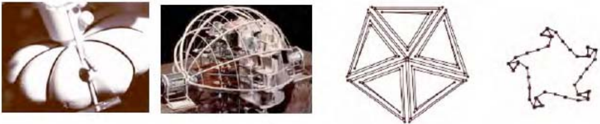
Figure: Preliminary brainstorming ideas of “Puffer Fish” like modules to incorporate inflatable (left), lightweight deployable (middle left), and mathematical origami principles (middle right, right) for a novel Extreme eXPeditionary Architecture systems analysis.
