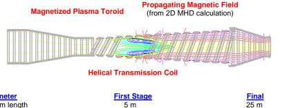
Parameter System length Plasma mass m<sub>p</sub> : Final plasma velocity: Acceleration (Force): Thrust Power (1 kHz rep) First Stage 5 m 0.2 mg D<sub>2</sub> 3x10<sup>5</sup> m/sec 2x10<sup>10</sup> m/s (4 kN) 9 MW
