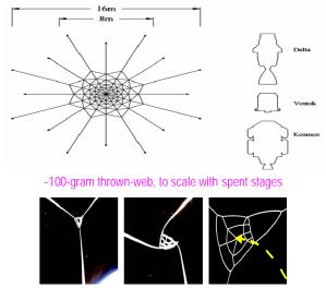
Net spin-up viewed from support, with desired payload trajectory shown in frame 3.
