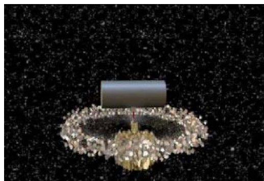
Figure 1: "Rock-breaker" plasma beam cutter generates a doughnut-shaped cloud of nominally 0.2m blocks.
