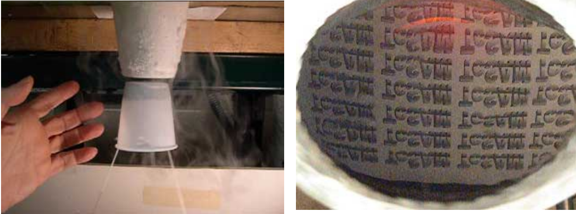
Figure 6. Model of spinning liquid mirror on a superconducting bearing by Professor Ma. (a) shows the bearing, with a nitrogen-cooled YBCO superconductor in the upper cup, and a neodymium magnet in the inverted cup below. The gap is \sim 3 mm. Hanging on 3 strings below is a 20 cm spinning dish of black soy sauce with \sim 8'' focal length (b). The lettering is the reflection of a screen above.
