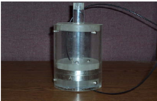
Figure 1: (a) Sketch of particle in liquid test vessel, (b) Picture of experimental apparatus.
