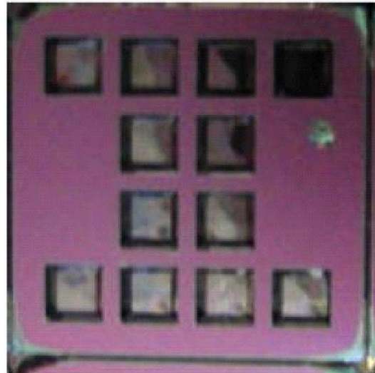
Figure 10: First-generation MEMS gate design showing the viewing windows etched into the bulk silicon. Each viewing window contains about 4 \times 10^4 emission channels. The current MEMS gate is a second-generation design.
