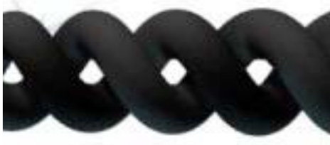
Figure 4-10 Proposed dual chiral nanotube bundle actuator. Aerospace Research Systems, Inc.
