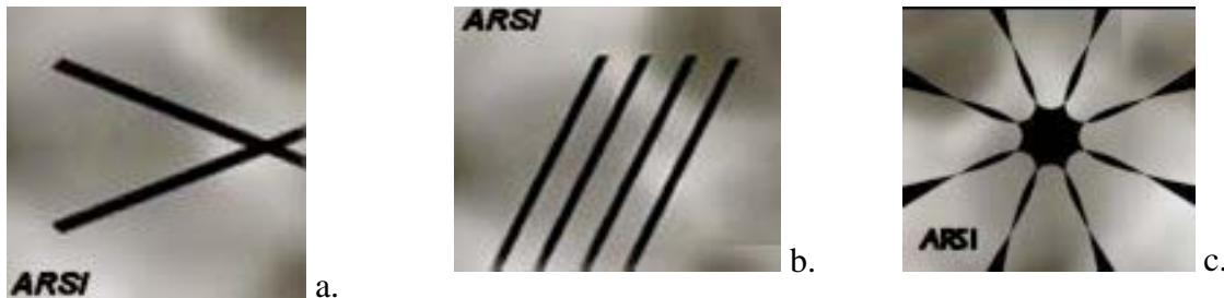
Figures 4-9: NiTi SMA conceptualized actuator configurations for thin film membrane structures; a-scissor induces expansion-contraction in a scissor motion force vectors resolving in two directions, b-herring bone providing expansion-contraction in a specific linear motion, c-aperture can be programmed to differentiate between two signals inducing either a rotational force or a liner-reducing motion where the actuator arms shorten. (ARSI Systems Engineering Laboratory, Cincinnati, Ohio)
