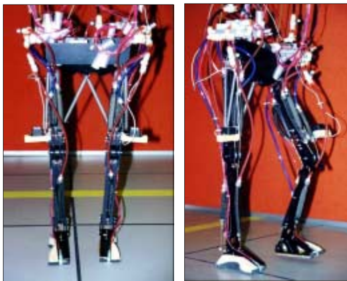
Figure 12. Prototype of the biologically inspired legged IIS Bio-Bot (April 1999). Sensors were attached to each thigh. A three dimensional hip joint was added to provide smooth transitions from one leg to the other during walking. Springs (to be replaced by muscles) were added to constrain the excessive movement of the new 3-D hip joint. A new foot design was added to provide smooth rolling motion during walking. In the right picture the robot is standing on one leg , i.e. the right leg.
