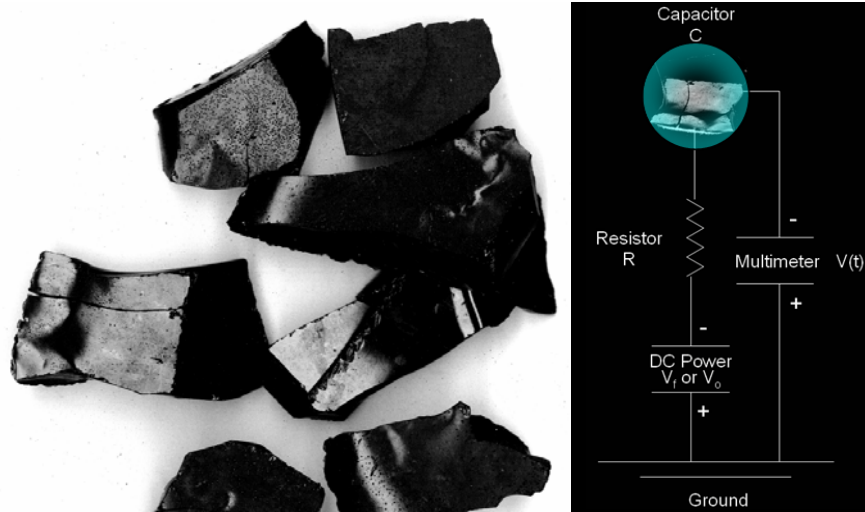
Figure 8. Carbon Nanofoam Samples and Schematic of Test Setup
