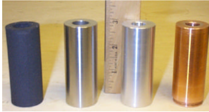
Figure 25: Tubes of Various Materials used in Preliminary Testing From left to right: YBCO superconductor, stainless steel, aluminum, and copper
