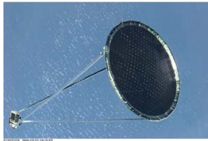
Figure 4. 14-meter L'Garde Inflatable Antenna Space Shuttle Experiment.
