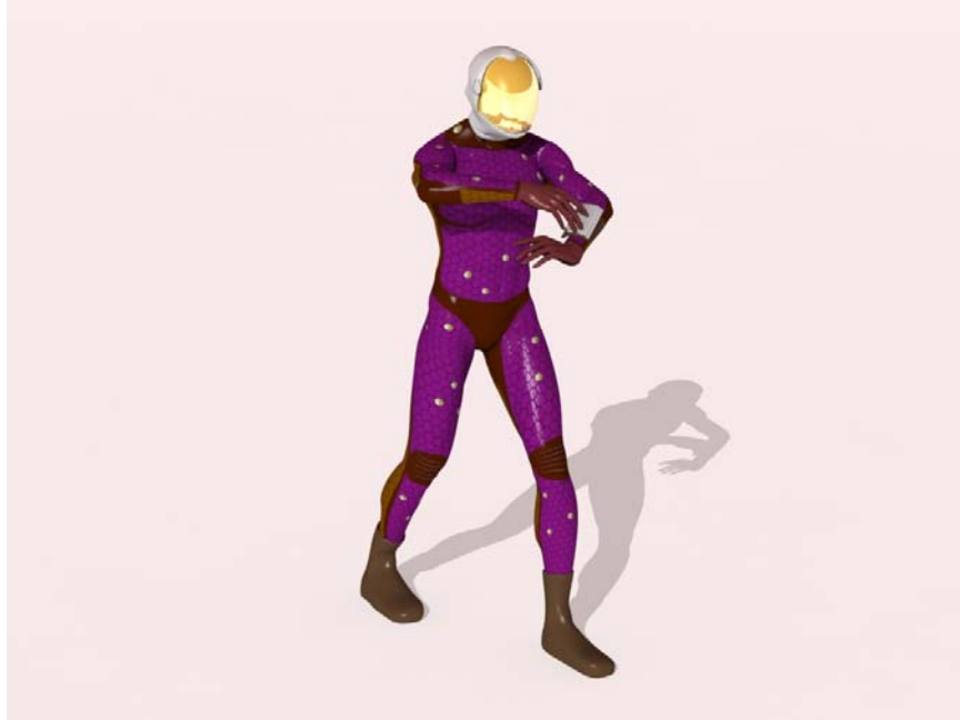
Figure 18: A space suit, modeled after the Biosuit , covered with a power skin and sensors. Sensors can be placed at random on the suit and draw power from the skin itself. (image by Chris Lund © IntAct Labs)
