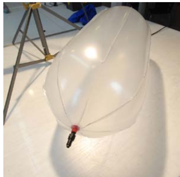
Figure 16. Fully inflated lightweight structures (side view and end view) indicating seam pattern.
