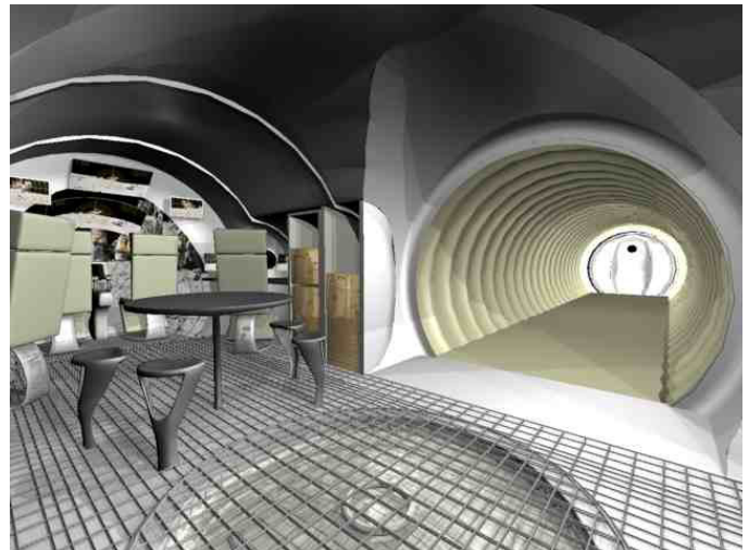
Figure 42. MSR Scorpion, interior view of the deployed inflatable environment doubling the volume of the MSR.
