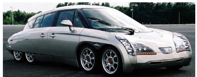
Figure 58. Ellica Electric car 230 mph, 185 miles range at lower speeds before recharging batteries.
