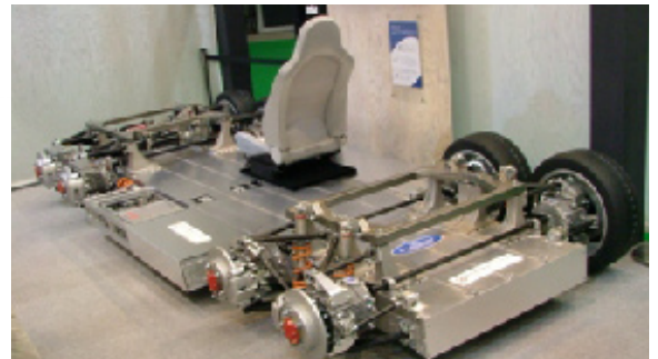
Figure 55. Ellica 8 wheel drive train with independent electric motors.
