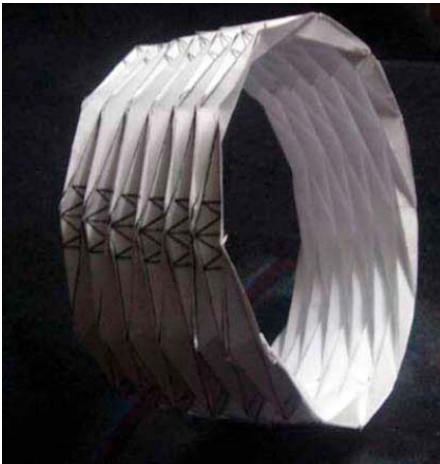
Figure 17. Origami hexagon (6-sided) folded structure model.
