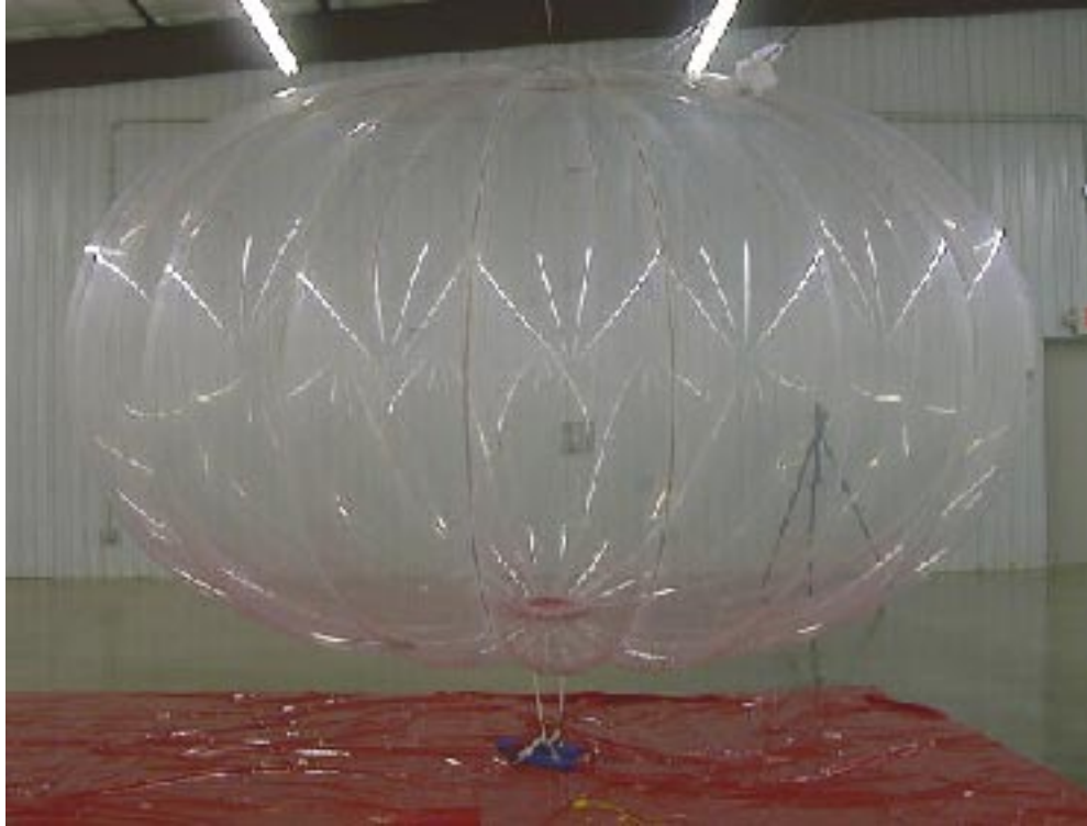
Figure 1.3 ULDB Scale Model Polyethylene Pumpkin Test Balloon
