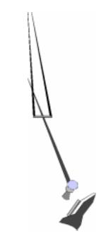
Figure 14. Tillotson Two-Tier Tether
