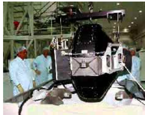
Figure 3-2. Control Moment Gyro for the International Space Station
