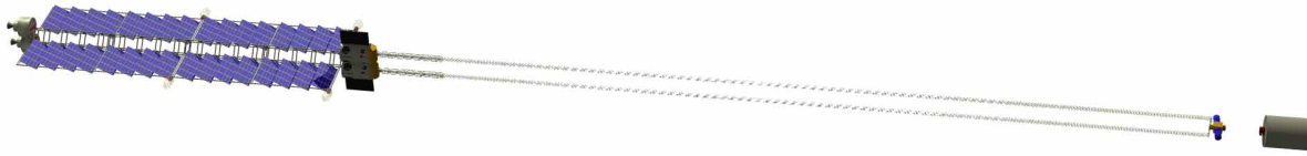
Figure 5. Tether Boost Facility with two modules, capable of tossing 5000 kg to GTO and 2000 kg to LTO. (Tether length not to scale)
