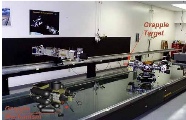
Figure 3. The LLNL microsatellite AR&C test facility, suitable for the GRASP experiment.
