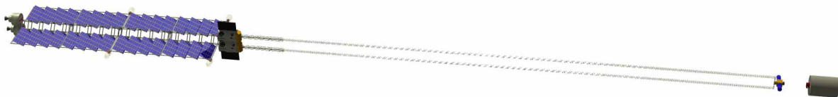
Figure 7. Tether Boost Facility with two modules, capable of tossing 2000 kg to LTO. (Tether length not to scale)
