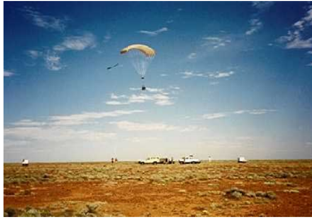
Figure 4-15. IST Aerospace GPADS-Light during qualification testing
