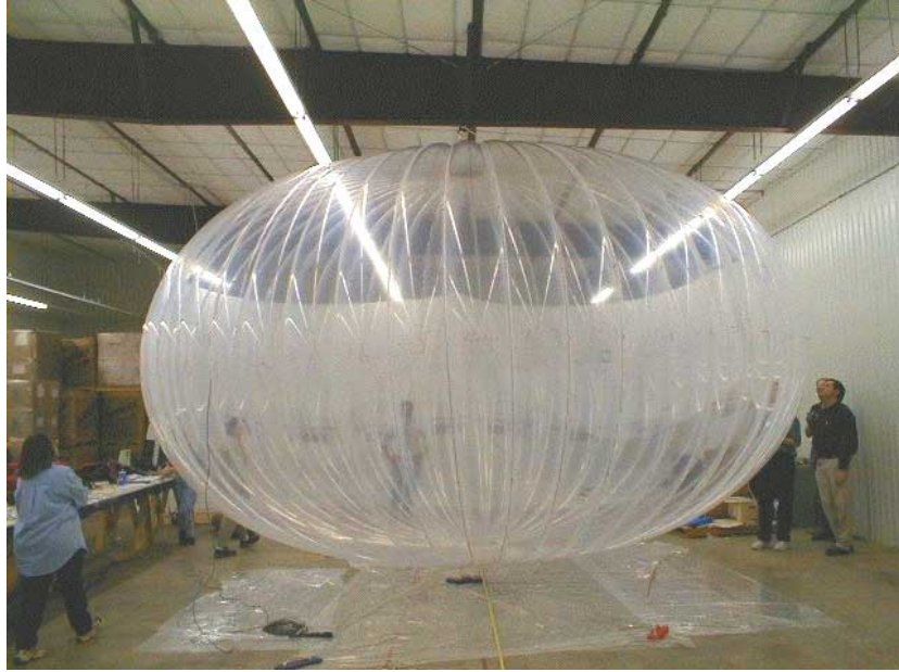
Figure 1-3. ULDB Envelope Test Showing Its Characteristic Shape
