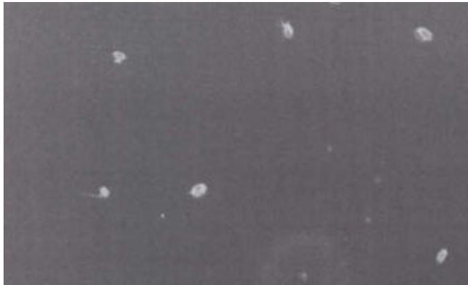
Figure 11. Plan view scanning electron micrograph of melted JSC1 surface
