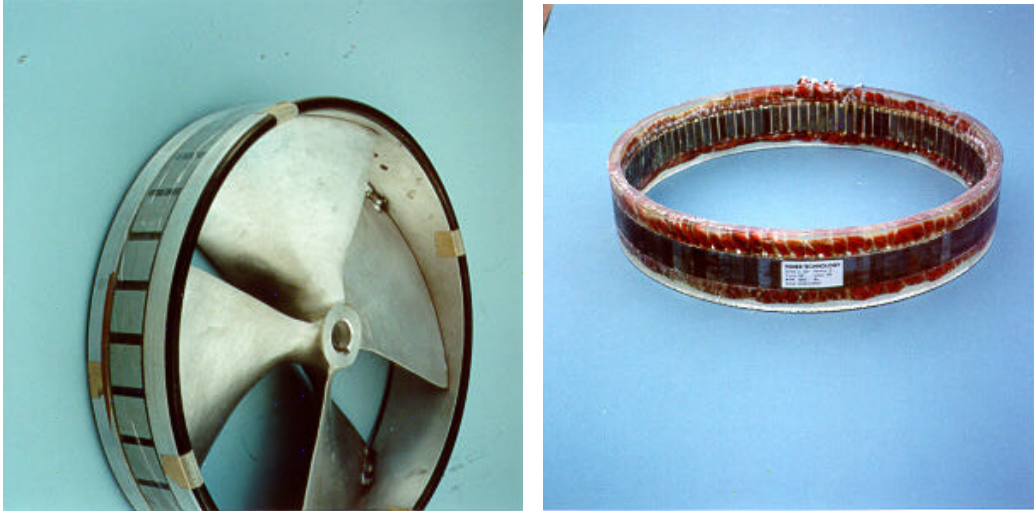
(a) (b) Figure 2.9 Toroid Rotor Components (a) Rotor, (b) Coil
