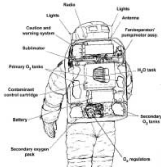
Figure 20. The EVA life support system backpack can interfere with heat rejection from the suit surface or offer additional heat rejection opportunities.
