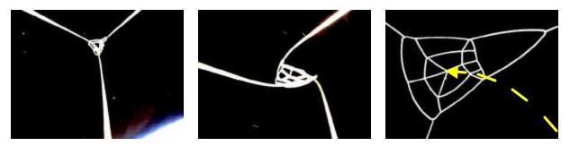
Figure 6. Net spin-up viewed from support, with desired payload trajectory shown in frame 3.
