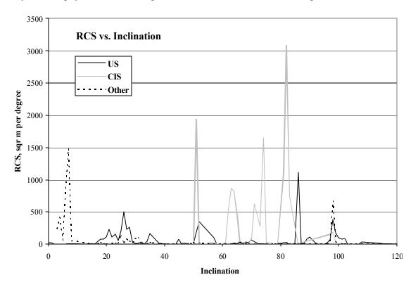
Figure 1. Total Radar Cross-section (m2) vs Inclination for Objects in Low Earth Orbit
