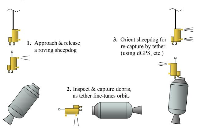
Figure 7. Two-stage Cooperative "Two-Dog" Capture of Passive Objects by Tether
