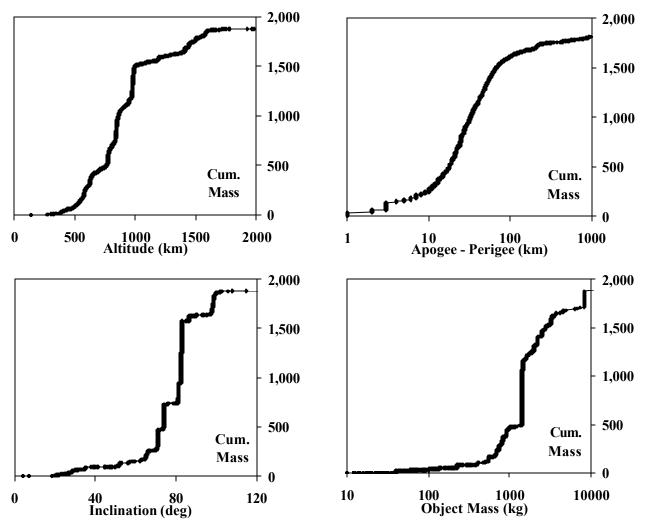
Figure 2. Key characteristics of >5 kg debris objects in low earth orbit
