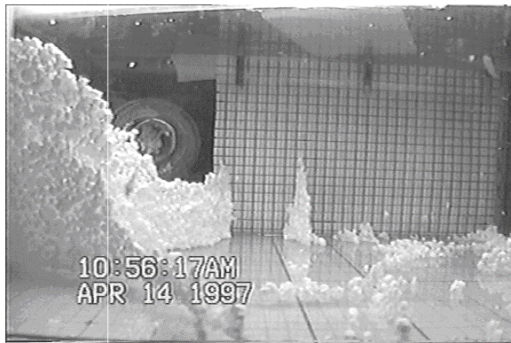
Figure 4.5 Walls of Styrofoam particles form in an acoustic resonator operated at its 110 mode. Reduced-gravity flight test, April 1997.
