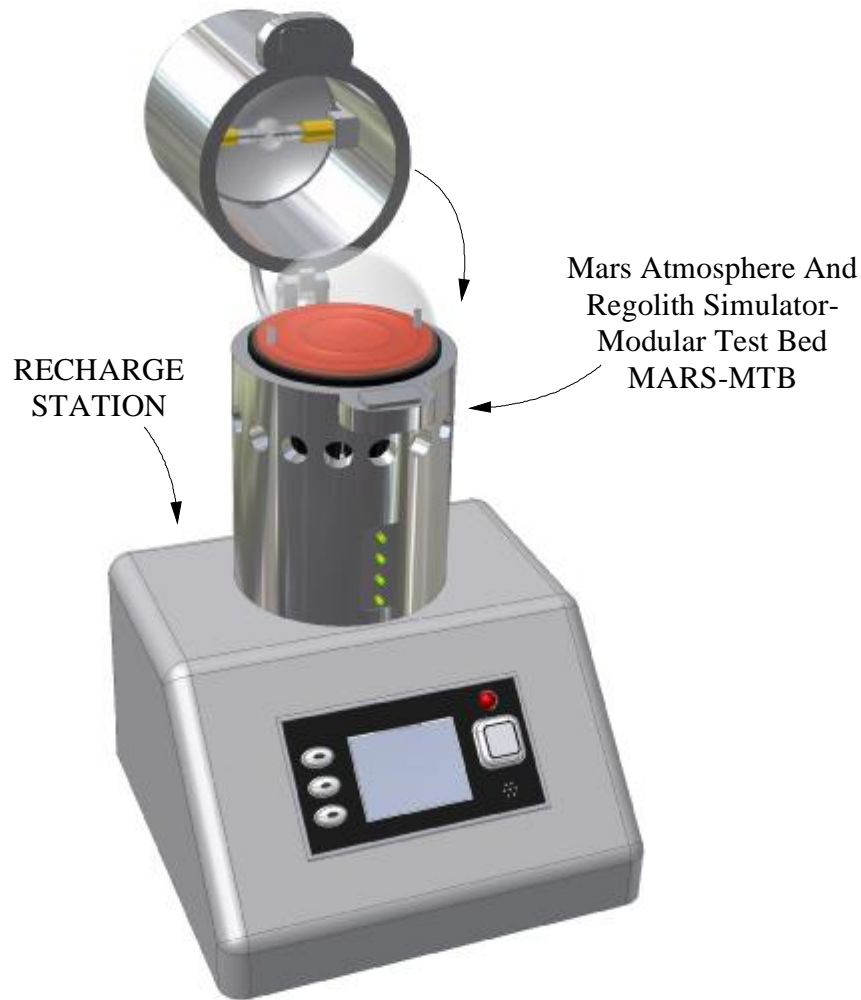
Figure 17. Three-dimensional overview rendering of the MARS-MTB. The diameter of the regolith component (red) is 2.7" (6.9 cm). Volume under the dome is 84 cm 3 .
