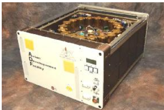
Figure 3. Spaceflight hardware for fundamental biology built by SHOT for NASA – “Avian Development Facility” – with 32 adaptable variable-g centrifuge positions for specimens
