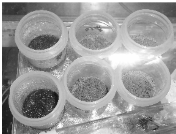
Figure 7. Differences in sample moisture. By the end of each experiment, samples located toward the ends of the chamber (left) contained more water than samples in the middle of the chamber (right). Sample jars were arranged such that each triplicate series experienced the full range of moisture within the simulator chamber. The culture tube at the bottom of the figure was for another experiment running simultaneously.
