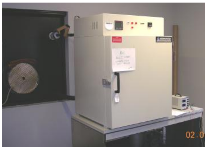
Figure 11. Thermal chamber installed on reinforced support and connected to LN 2 inlet from the outdoor tank and exhaust to the outdoors. The disk-shaped object at the left is the safety exhaust fan that is actuated by the low-O 2 sensor that has been installed and tested. The fan can also be switched on manually for room air control.
