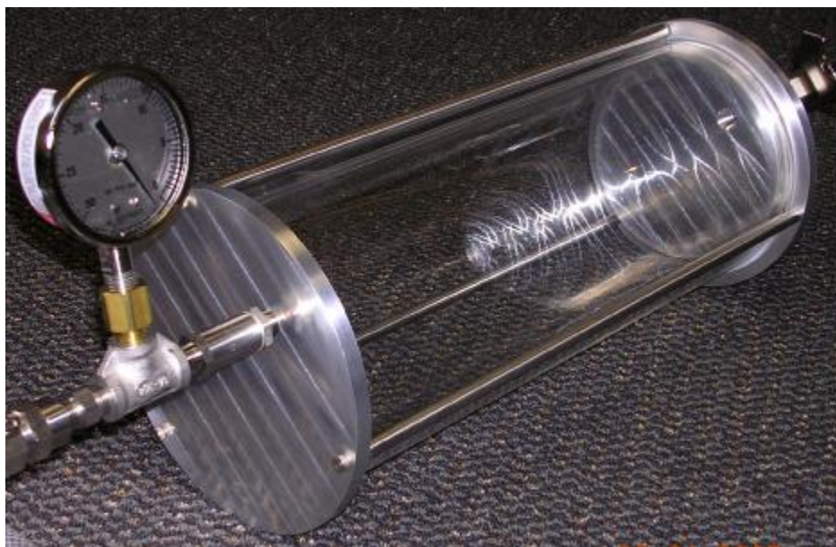
Figure 15. Photograph of quartz cylinder fitted with end-plates, gaskets and inlet and outlet fittings and vacuum gauge. The cylinder is approximately 45 cm long and has a volume of approximately 5.6 l. In normal operation the vacuum gauge is outside the thermal cabinet.
