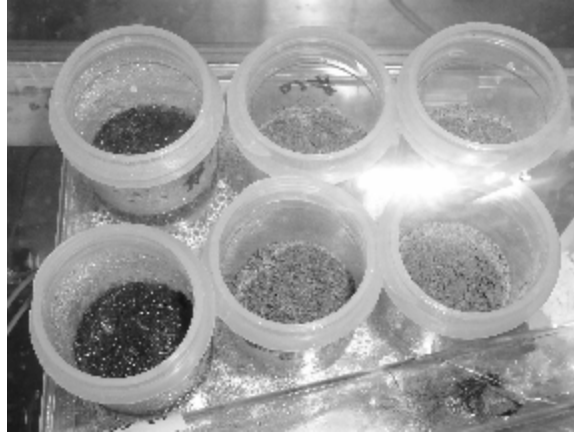
Figure 34. Differences in sample moisture. Examples of 25 ml polypropylene jars containing samples at the end of an experiment. By the end of each experiment, samples located toward the ends of the chamber (left) contained more water than samples in the middle of the chamber (right). Sample jars were arranged such that each triplicate series experienced the full range of moisture within the simulator chamber.
