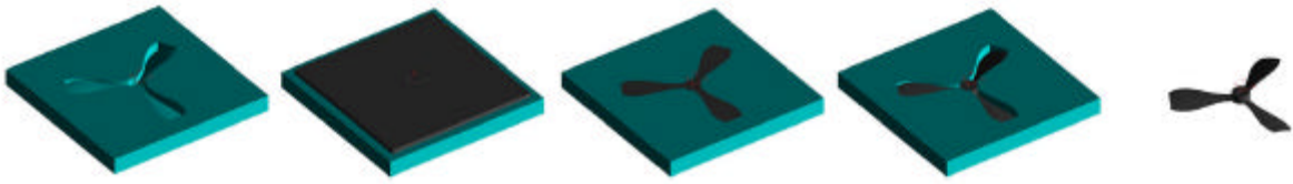
Figure 14. Rotor fabrication steps 1 to 5
