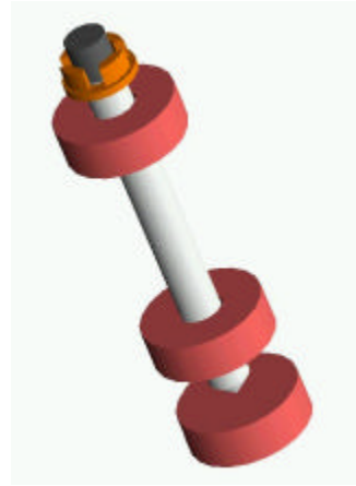
Figure 21: Experimental jewel bearing setup
